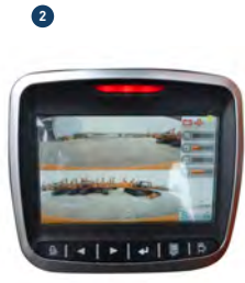
360-degree vision is provided in real time through computerized images from 5 cameras.
