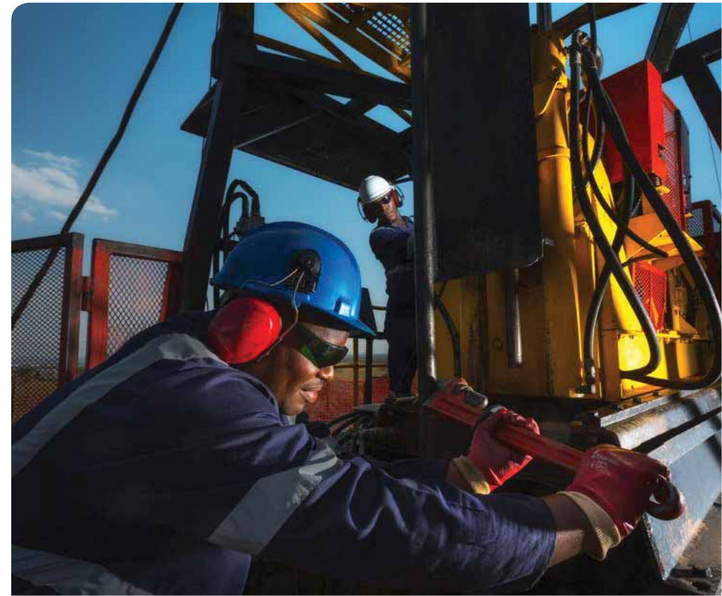
Employees wearing the type of noise prevention equipment required in an environment where the noise level is above 85 decibels
