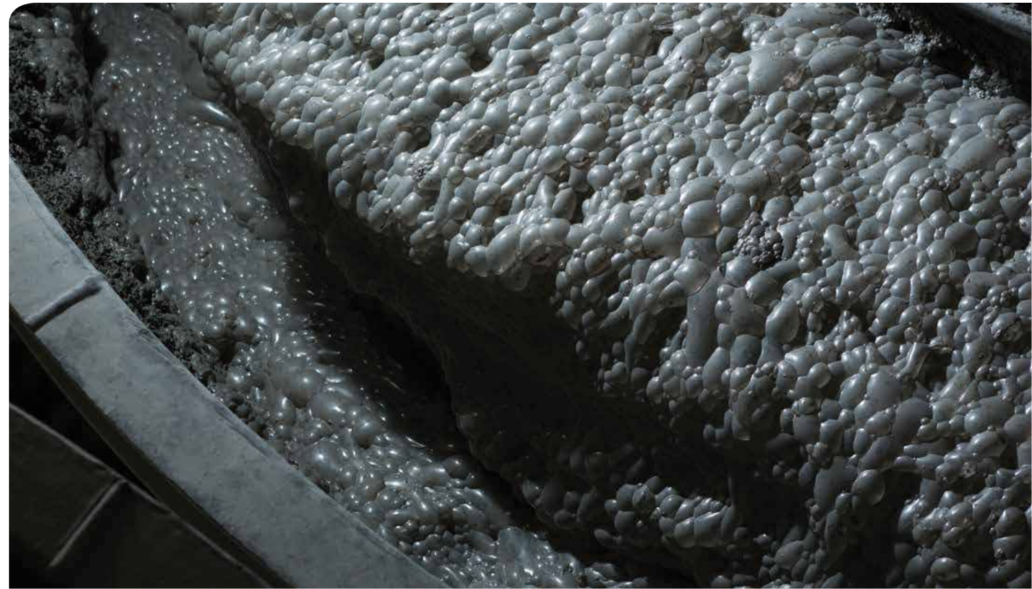
↳ The flotation process in the RBPlat concentrator
