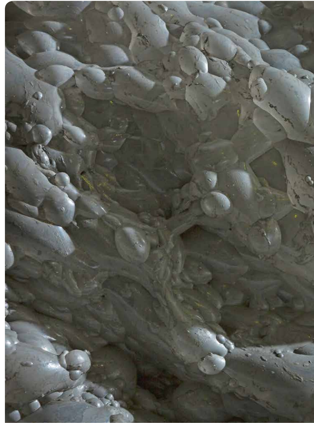
The froth produced as part of the flotation process in the RBPlat concentrator
