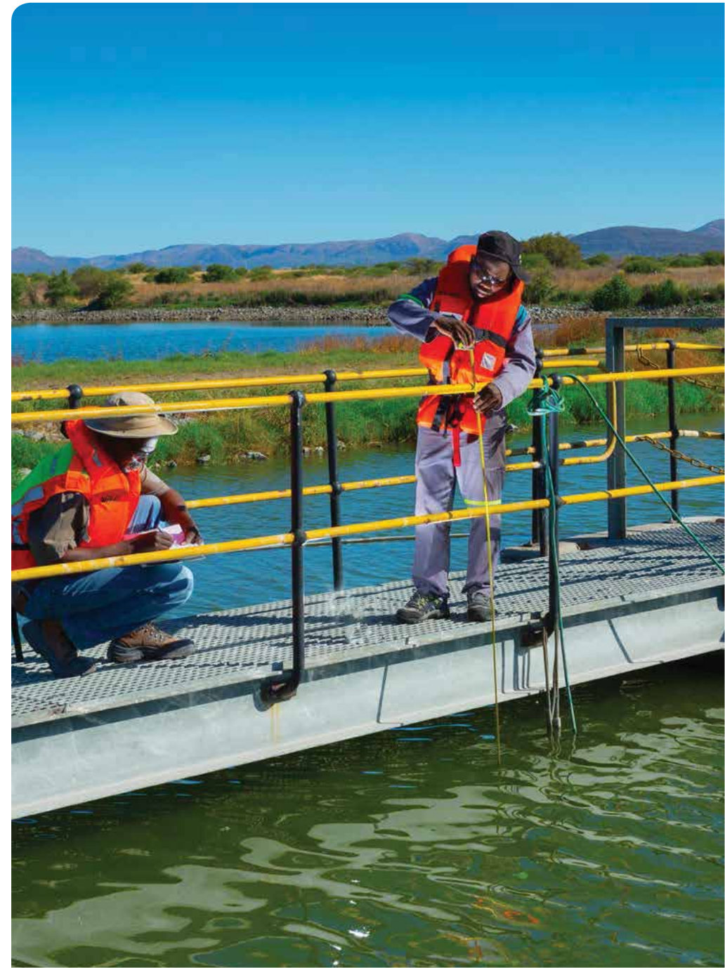
The Fraser Alexander team measuring the levels of the return water dam at BRPM
