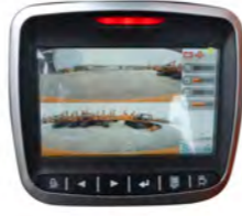
360-degree vision is provided in real time through computerized images from 5 cameras.
