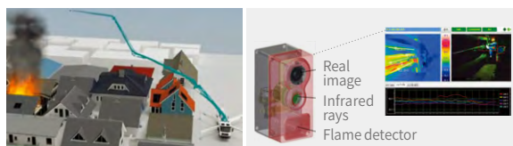
Unmanned flexible fire apparatus (boom length: 60 m)
