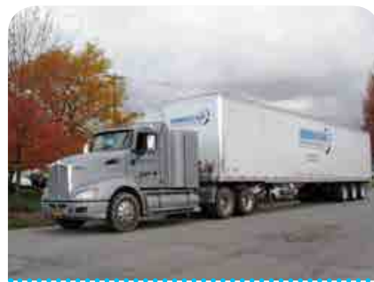
△ Tri-axle trailers increase load, reducing trips and associated GHG emissions.
