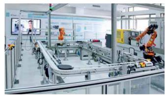
In the Application Center for Automation Technology at the CDHAW (Chinese-German University of Applied Sciences) at Tongji University in Shanghai, instructors and students work intensively on the individual and overall functions of a complete production plant with robotics and CNC technology, including networking, visualization, and automation technology.
