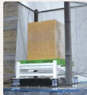
Collapsing cargo from shaking (above). Confirming the effects of various methods for prevent collapsing using film and installing rubber stoppers
