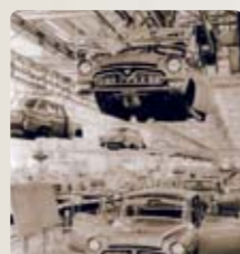
1959 Chain conveyor system installed in Japan's first passenger automobile factory
