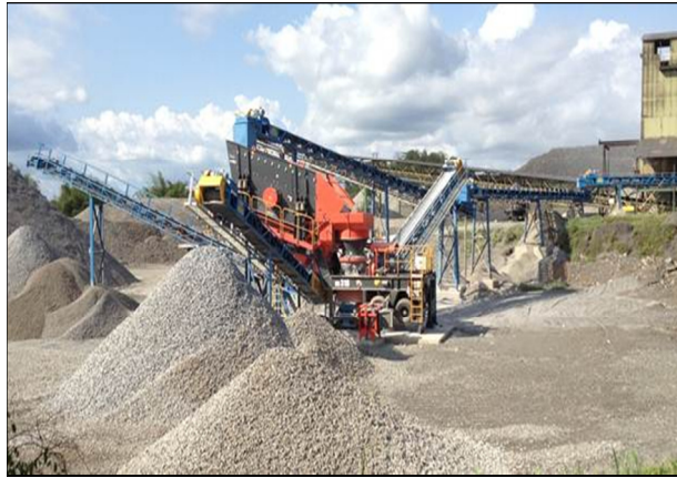
Plates 12 and 13: LAYOUT – transfer point from primary section to US 316 mobile unit
