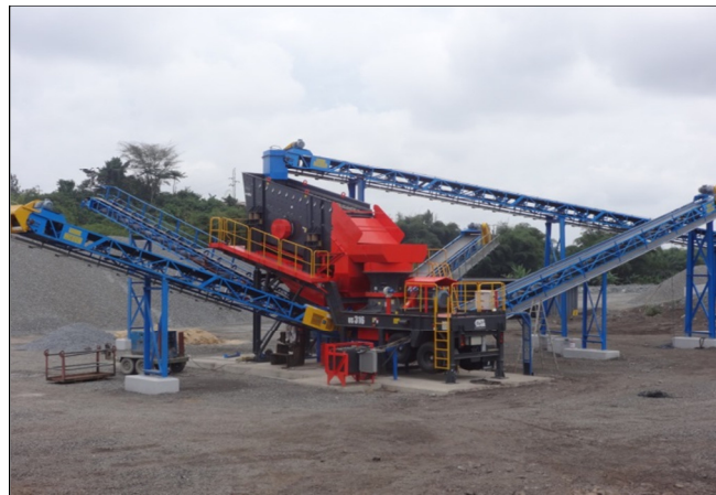
Plates 10 and 11: CPE – Foundation and installations – US 316 PLANT and US 316 Mobile unit with all conveyors connected
