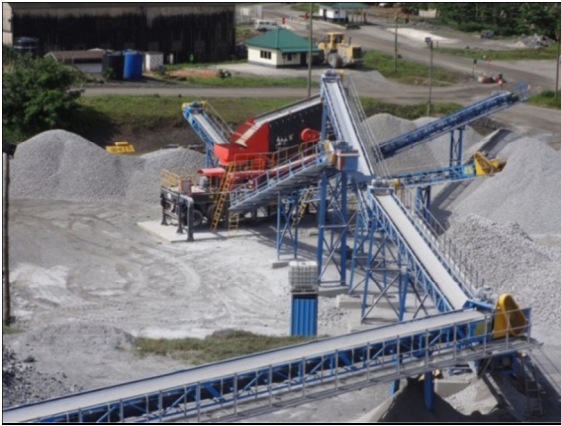
Plates 12 and 13: LAYOUT – transfer point from primary section to US 316 mobile unit
