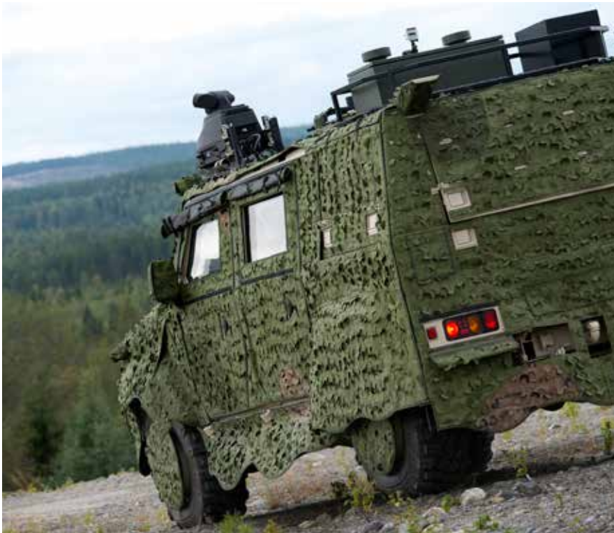
Mounted on the roof of an off-road vehicle, Saab's warning system can detect Chemical, Biological, Radioactive and Nuclear threats (CBRN).
