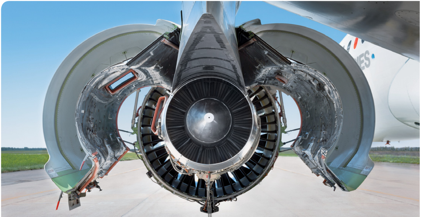
Eco-efficient engine: Geared Turbofan in new Bombardier CSeries before its maiden flight.
