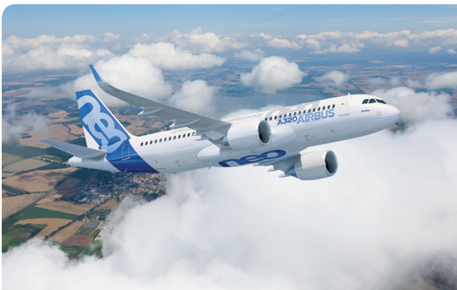
An A320neo powered by PW1000G engines will emit around 3,300 tons less CO 2 every year.
