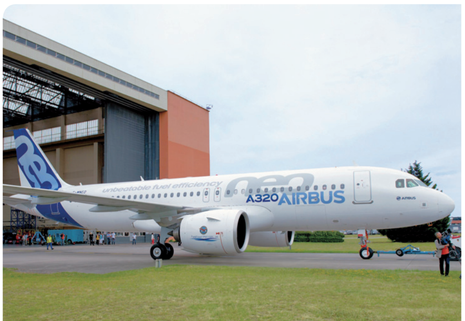
Through the use of the geared turbofan engine, fuel consumption and hence CO 2 emissions will be reduced by as much as 15 percent.
