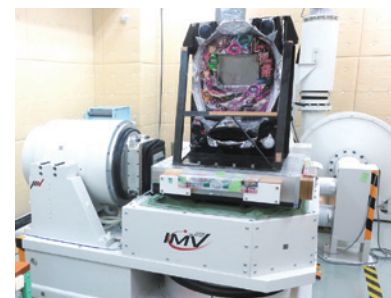
Anticipating vibration during product shipping, we use vibration testing machines to check durability and other such aspects.
