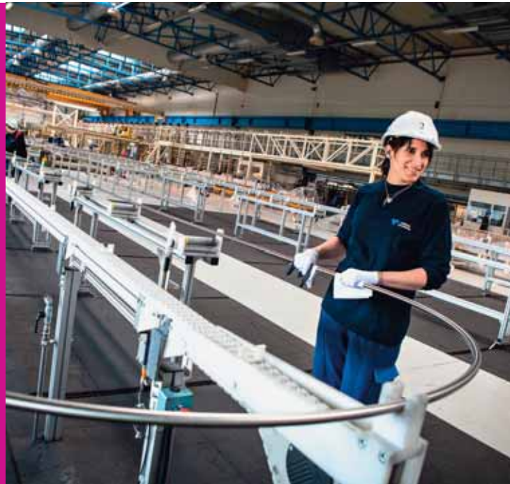
↑ Welded tubes for heat exchangers are used in power generation, desalination and process applications.
