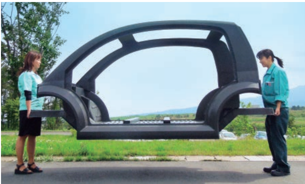
Structure of concept car made using CFRP
