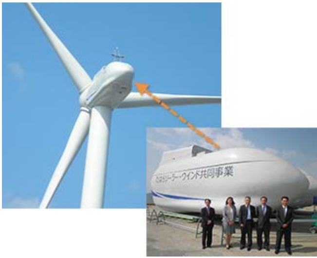
The downwind turbine with blades (left) and nacelle before installation (right) (pictures taken April 2014)
