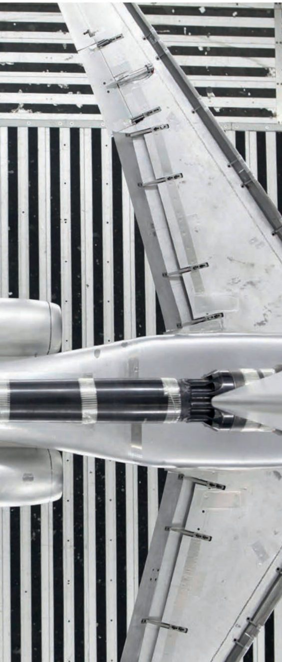
Wind-tunnel testing of the Falcon 5X With "flaperons" on its wings, the Falcon 5X offers unrivaled performance.
