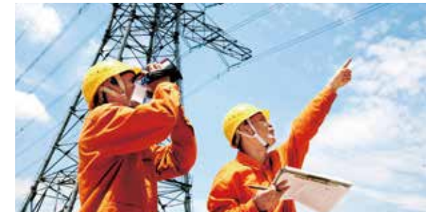
Using infrared devices to test facilities and investigate hidden dangers in the wild ▲
