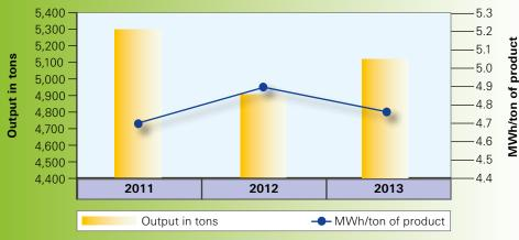
The energy consumption indicator shows the relationship between the total consumption of the individual energy sources (electricity, natural gas, heating oil) and the total product output.
