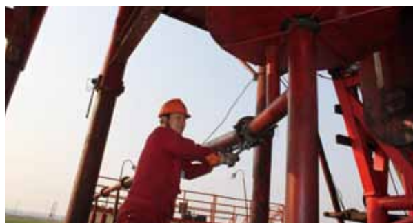
An operator from Sinopec Henan Oilfield is connecting workover fluid recovering pipeline. It was very difficult to recover workover fluids, which will pollute the well site if not recovered. The closed circular facility Henan Oilfield developed independently made it possible to direct workover fluids to mud tank via recovering pipeline
