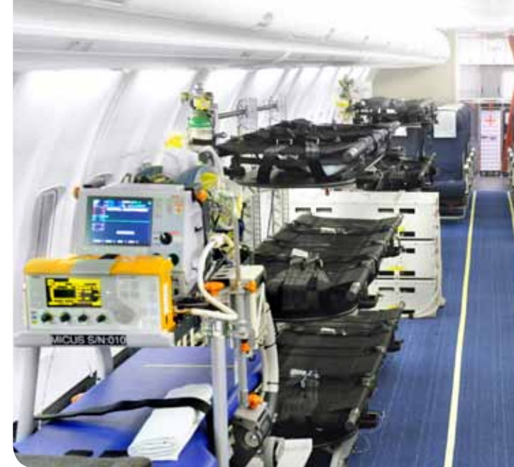
The interior of a Boeing 737-800 remodeled to enable advanced and simpler air ambulance transportation within the framework of SNAM.
