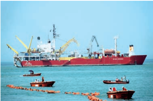
Traction Boat is drawing the floating-point package which holds the sea cable
