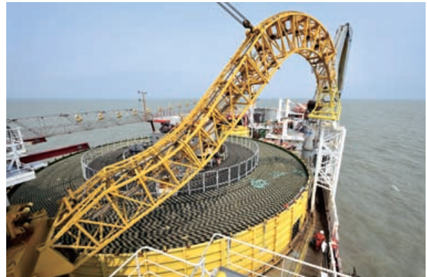
Over 100 km of 500 kV Cable is loaded on the ship
