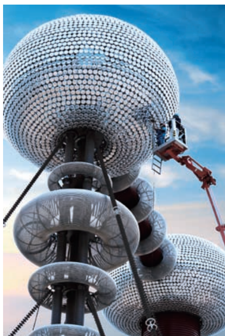
An Inspection on 2250kV Fundamental Frequency Testing Transformer
