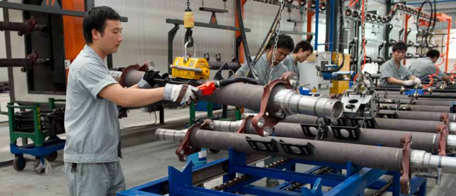
SKF supplies both seals and tapered roller bearings for trailer axles to Guangdong Fuwa Engineering Manufacturing Co. Ltd. in China, the largest trailer axle manufacturer in the world.
