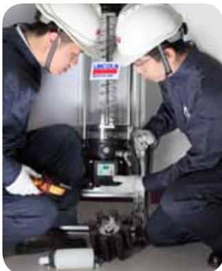
Installation of a Lincoln automatic lubrication system for a wind turbine.
