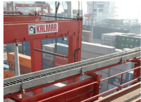
Evyap Logistics in Istanbul, Turkey, operates Cargotec's latest generation all-electric Kalmar E-One2 RTG cranes equipped with an energy saving power unit.
