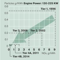
Nitrogen oxide and particulate emissions have fallen by about 60% since 1996. When Tier 3 was introduced, Volvo Construction Equipment launched products equipped with the new V-ACT technology (Volvo Advanced Combustion Technology), which minimizes emissions by adjusting the combustion process in the engine. Nitrogen oxide and particulate emissions will decline by a further 90% by 2014 compared with today's Tier 3 level.
