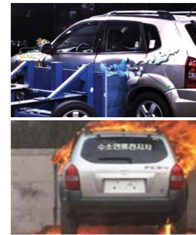
Collision Test of Hydrogen Fuel Cell Vehicle 1 Fire Test of Hydrogen Fuel Cell Vehicle 2
