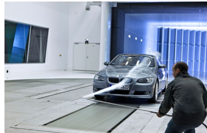
REDUCING CONSUMPTION WITH AERODYNAMICS — BMW Group wind channel.
