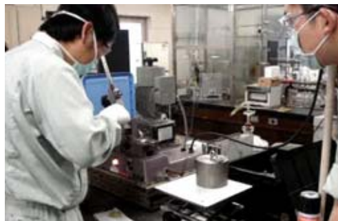
Risk assessment (friction sensitivity testing)
