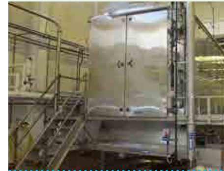
△ Steam and water recirculate inside to efficiently rehydrate beans.
