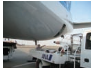
Wastewater removal by a water truck
