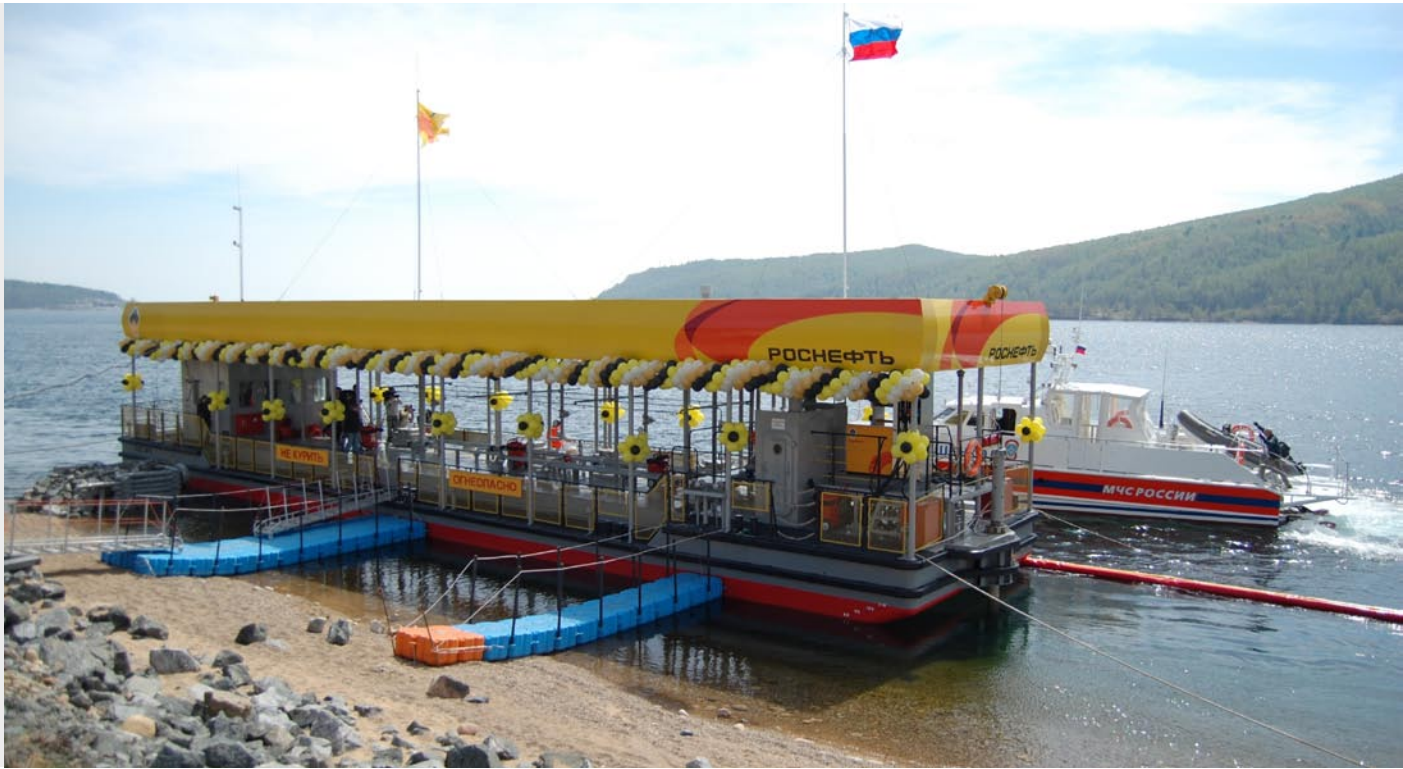
Floating filling station (river bunker) of Irkutsknefteprodukt
