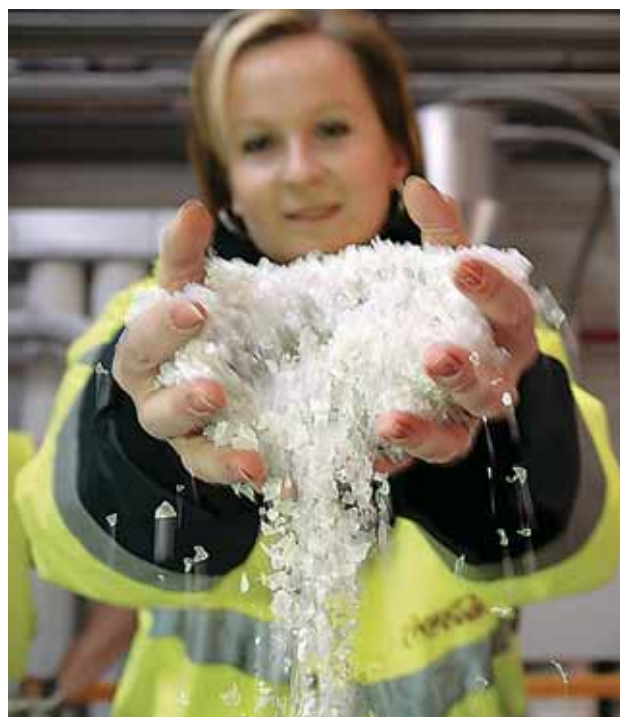
Recycled PET flakes from the PET2PET Austrian plant are mixed with PET pellets to produce preforms. The preforms are then blown into beverage bottles
