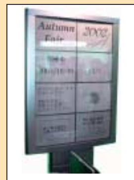
Figure 2: Low-Energy Consumption "Zero Display" Suitable as a Large Display Panel
