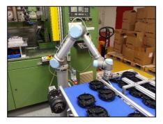
In the assembly area, we have installed two small 6-axis robots. One robot (left) was installed at a specialized milling machine for pick and place of the parts in and out of the workstation for machining. The other robot (below) was installed in the printing area where it also handles pick and place of parts in and out of fixtures of 5 different printing machines.
