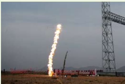
Short-circuit grounding experiment on the construction site of UHV AC pilot project
