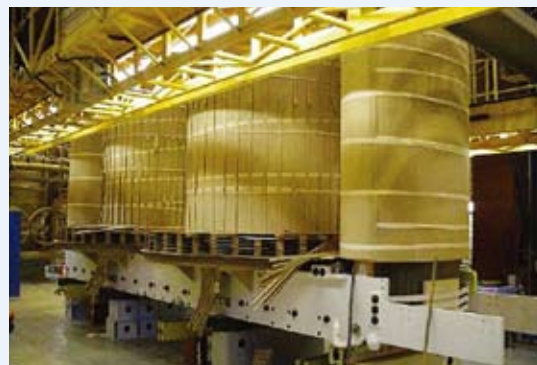
The factory assembly of the first transformer for Fengxian Station, Xiangjiaba - Shanghai \pm 800 kV UHVDC Demonstration project.
