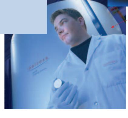
RS90 (Rapid Coating) is an ultra-high-performance Balzers system designed for mass-coating large batches of components, like parts for the automotive industry. Coatings with diamond-like hardness make longer-lasting, more reliable engines.
