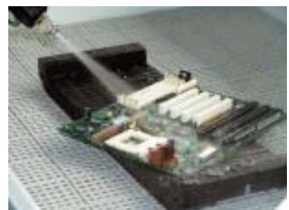
Example of water-blasting recovery of damaged equipment
