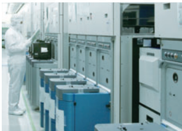
Clean room in a semiconductor factory that minimizes energy consumption using a local air conditioning system
