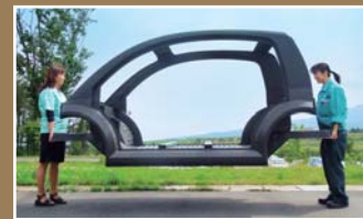
Structure of concept car made using thermoplastic CFRP
