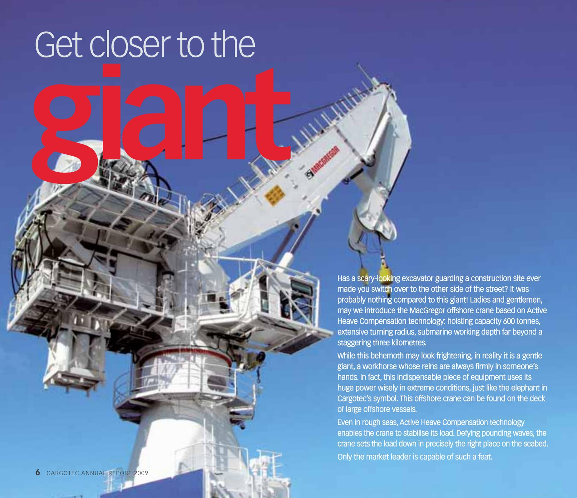
Has a scary-looking excavator guarding a construction site ever made you switch over to the other side of the street? It was probably nothing compared to this giant! Ladies and gentlemen, may we introduce the MacGregor offshore crane based on Active Heave Compensation technology: hoisting capacity 600 tonnes, extensive turning radius, submarine working depth far beyond a staggering three kilometres.
