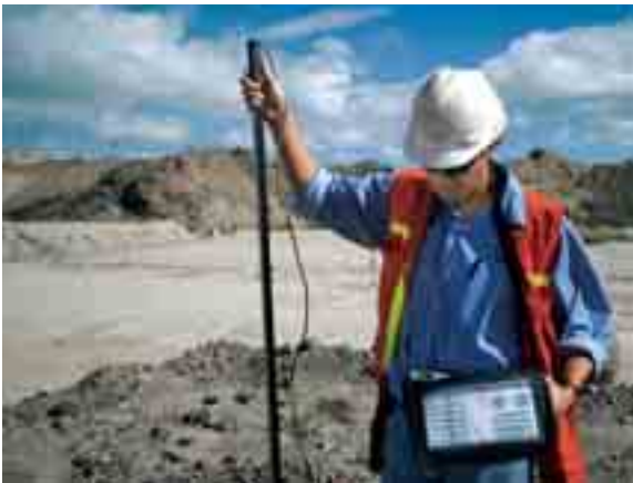
Environment Official Gabriel López Vazques manually measuring temperature and moisture levels in tailings and capping material.
