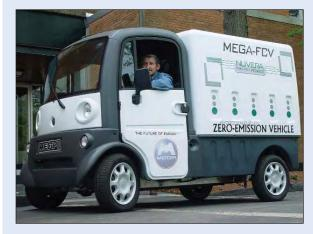
Fuel cell powered zero emission vehicle.
