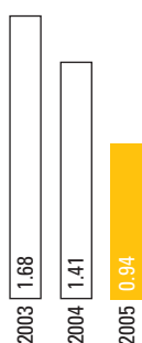
PRIMARY METAL FLUORIDE EMISSIONS RATE in kilograms per tonne of hot metal produced
