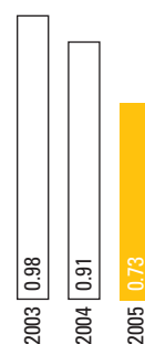
PRIMARY METAL PAH EMISSIONS RATE (Söderberg smelters only) in kilograms per tonne of hot metal produced
