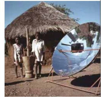
Solar cooker SK14 from EG Solar made from parabolic-shaped aluminium mirror sheets in Zimbabwe
