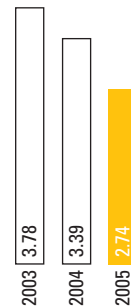
PRIMARY METAL PARTICULATE MATTER EMISSIONS RATE – SMELTERS ONLY in kilograms per tonne of hot metal produced
