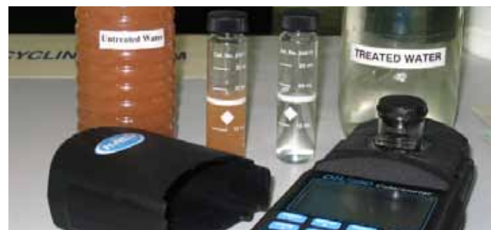
Based on Singapore's legislated code, the water discharged to public waterways must not exceed a TSS level of 50 mg/litre. CDL's effective silt and earth control measures have helped to achieve a remarkable TSS of between 10 and 15mg/litre for treated water discharged into the waterways
