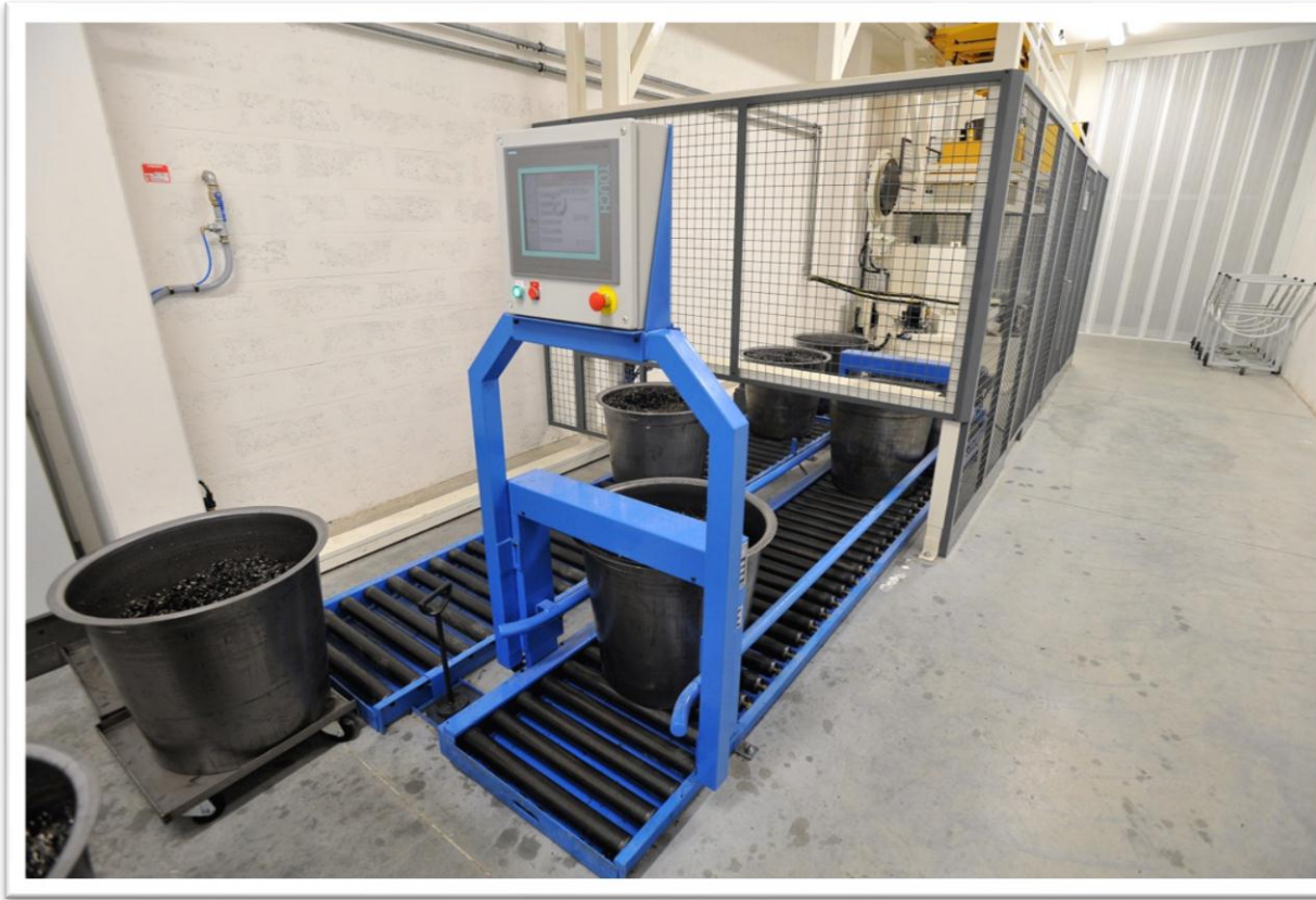
A machine which can clean forging shavings at Cejc
