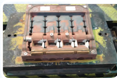
Iron based coated sand castings with core
