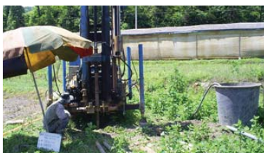
A scene of investigating soil contamination (drilling investigation)
