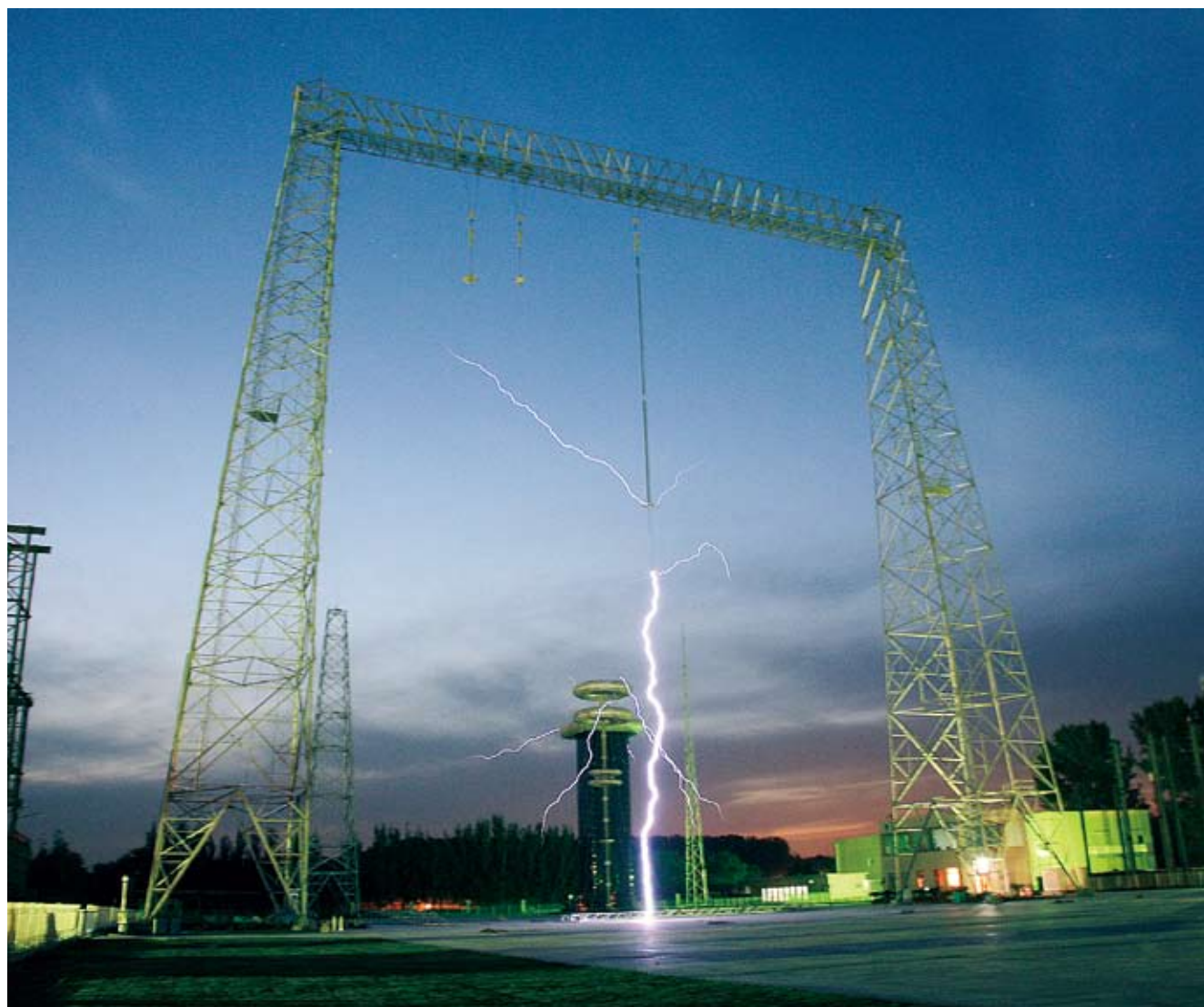
The output voltage of 7200 kV impulse generator at UHV DC Test Base creating the world record
