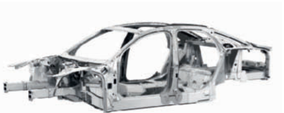
Audi Space Frame technology saves up to 40 percent in body weight.
