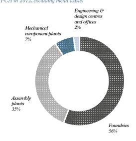
Due to the nature of their operations, the Charleville and Sept-Fons foundries alone accounted for more than half of total waste volumes, or 78 kg per vehicle. Most of this waste is spent foundry sand, much of which is recycled internally after on-site regeneration.
