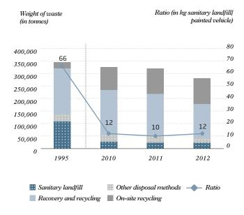
Improved on-site waste management systems have considerably increased the percentage of waste that is recovered or recycled, resulting in a 78% reduction in landfilled waste between 1995 and 2012. Much of this progress has been driven by the on-site reuse of spent foundry sand, which has increased fivefold over the period.
