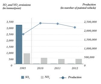
Since 1995, the gradual replacement of conventional high-sulphur fuel oil with low-sulphur fuels and natural gas has helped to
