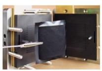
Membrane electrode assembly (the sheet shown at the center of the photo)
