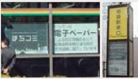
Left: Large-size electronic-paper signage at Toshima Post Office Right: Electronic-paper signage mounted on a bus stop sign at Higashi Ikebukuro 2-chome
